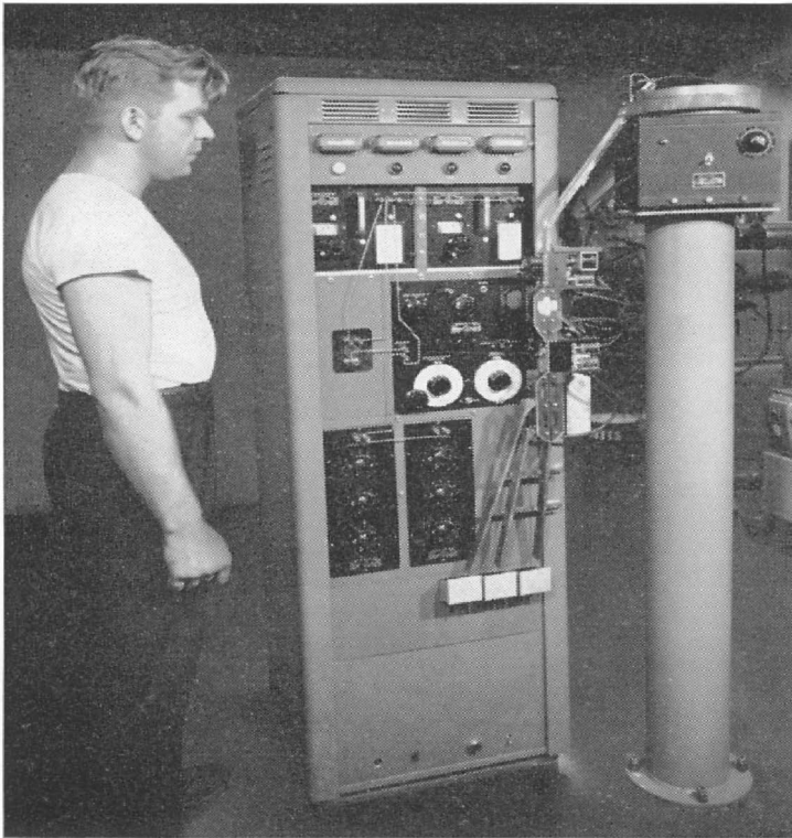
Figure 3. PROJECT TINKERTOY is the code name assigned to a program conceived and developed by the National Bureau of Standards for the Navy Bureau of Aeronautics, which involved the Modular Design of Electronics (MDE) and the Mechanized Production of Electronics (MPE).
