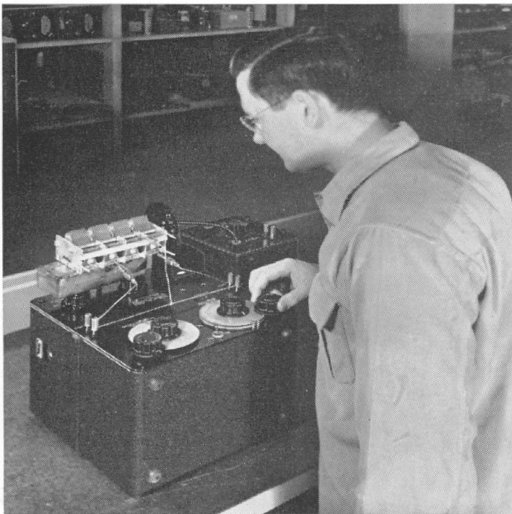
Figure 6. Another application in our own plant: testing and adjusting four-gang capacitors for proper tracking. The bridge is also used in the adjustment of ganged potentiometers.
