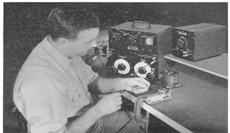
Figure 5. The Comparison Bridge used in adjusting an air-core inductor to 0.1% tolerance at General Radio's West Concord (Mass.) plant.
